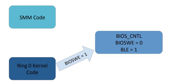
Here the attacker tries to set the BIOS Write Enable bit to 1 to allow him to overwrite the BIOS chip.
