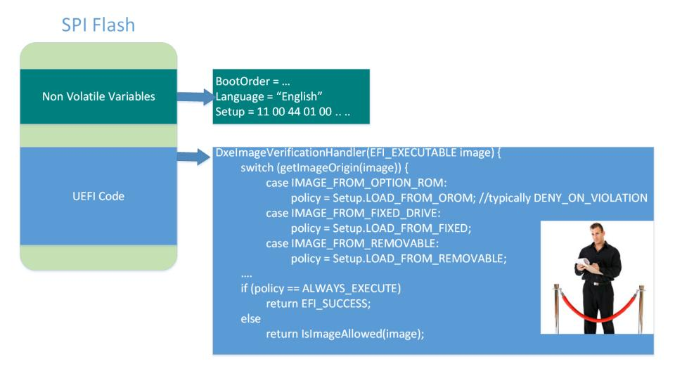
The EFI variables are typically stored on the SPI Flash chip that also contains the platform firmware (UEFI code).
