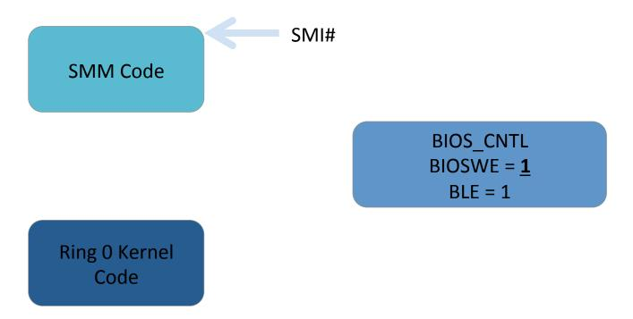
The write to the BIOSWE bit while BLE is 1 causes the CPU to generate a System Management Interrupt (SMI#).
