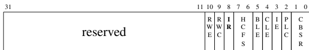
Figure 4. HcControl register. Bit 8 is the interrupt routing (IR) bit that determines how interrupts generated by events are routed. When clear, interrupts are routed normally on the host bus. When set, an SMI is triggered instead. The HCD uses this bit to indicate HC ownership by the BIOS.
