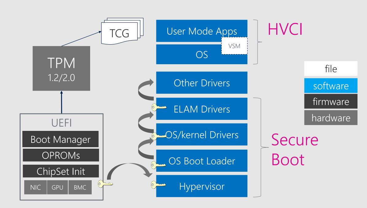
Secure boot currently uses static root of trust – OEM firmware included in attack surface
