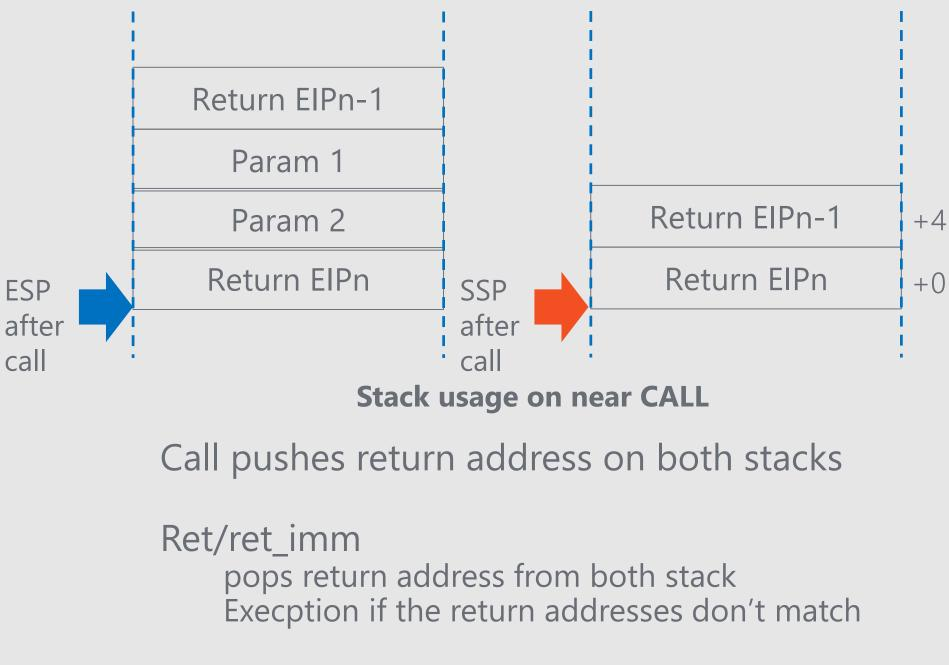
No parameters passing on shadow stack
