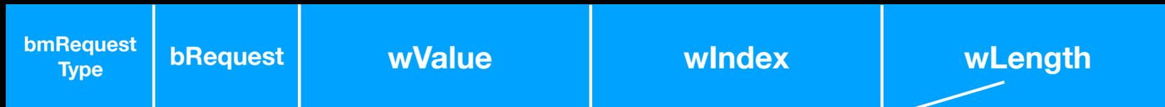
If wLength is non-zero, the setup packet is followed by a “data phase”, which e.g. in DFU mode is how the data is transferred from host to device, although this can also be done device-to-host depending on the bmRequestType
