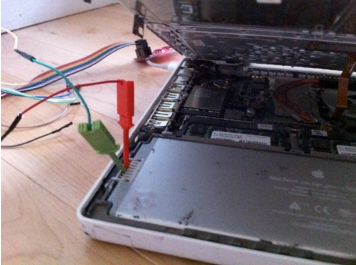
Figure 10: Sniffing the battery to host communications
