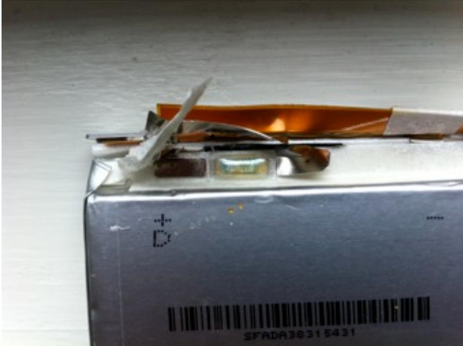
Figure 8: Here is a MU092X Thermal cutoff.
