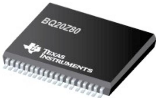
For Apple laptop batteries, the main component is the bq20z80 Gas Gauge (or similar model). This component interacts with the host via SBS data over SMBus. It has reprogrammable Flash Data as well as elements of the firmware itself can be changed.
