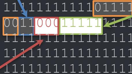
Freeing **Busy chunk** will coalesce with **3Q Chunk** and use overwritten **BackwardQ** of **12** joining **2Q chunk** with **7Q chunk**.
