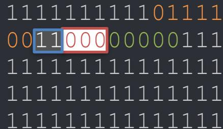
Due to **BackwardQ** being **12**. Freeing **5Q chunk** will read **BackwardQ** and add **7Q+2Q+3Q (12Q)** to free list whilst **chunk** still being by program.
