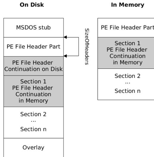
**Figure 3.10:** Dual PE File Header (referring to [VP11, slides 13, 14])
